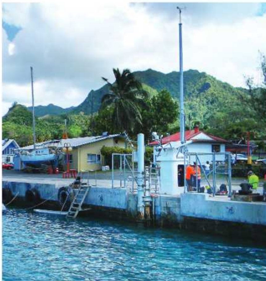
Figure 4. Technicians working on the Cook Islands tide gauge, which has been monitoring sea level and weather conditions in Rarotonga for over 25 years.
